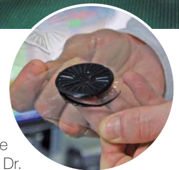
Test piece for a compound from the rheometer
